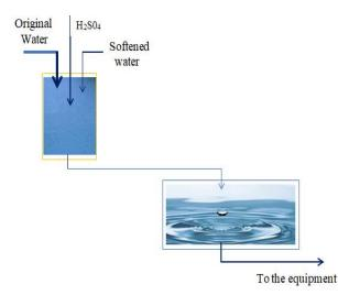
The upper tank was supplied with water from the water supply (W=12 mg eel/l) and softened water from the boiler room (W=0.1 mg eel/l). By mixing these waters in certain proportions, water of a given hardness was obtained. To neutralize the alkalinity of the water to the required level, sulfuric acid was supplied to the upper tank. Then the water was poured into the lower tank, which feeds the cocowinding equipment.
