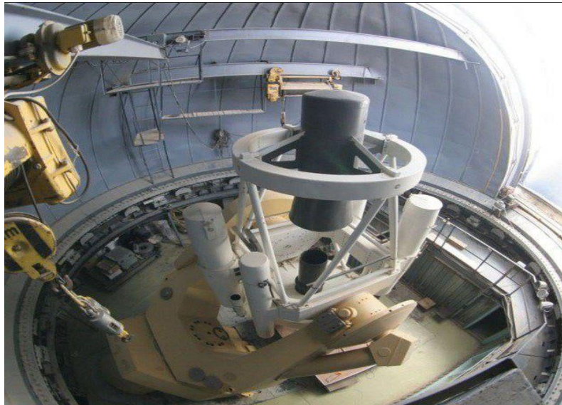
Pic.5. Reflecting telescope - AZT-22 with mirror diameter ( D = 1.5 m)
