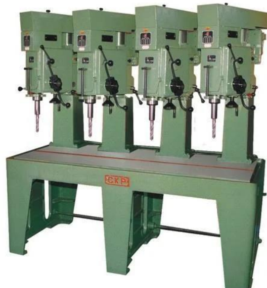
Fig 4: Gang Drilling Machine
