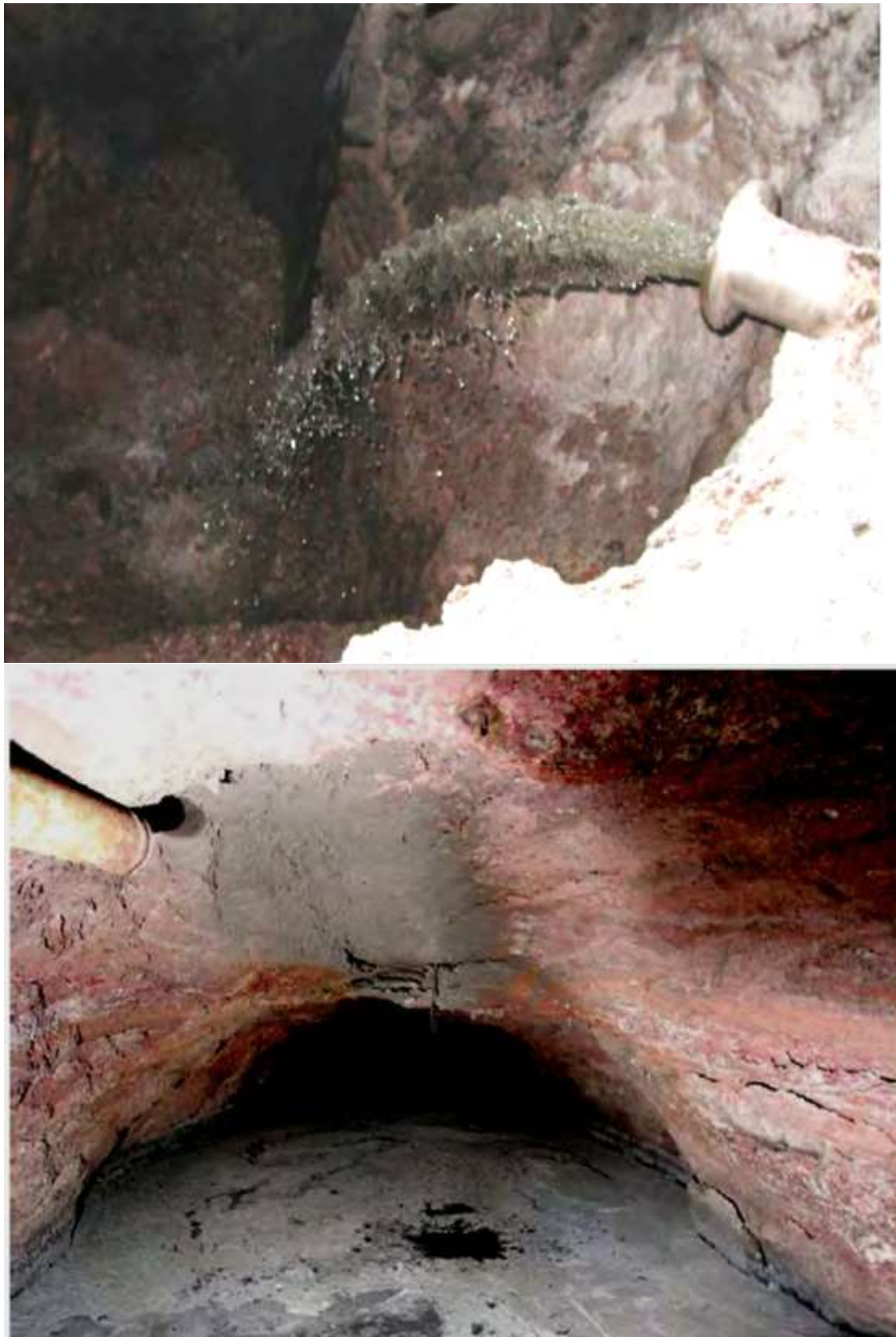
Fig. 3. The process of hydraulic laying in laying chambers
