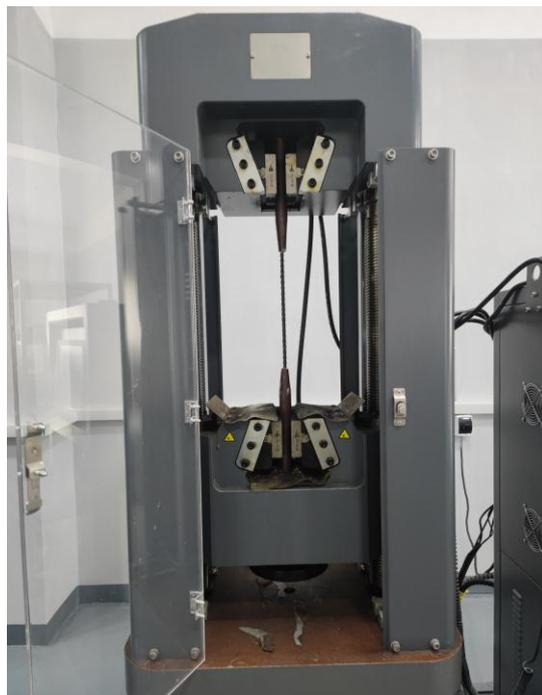
**Fig. 2. Testing BFRP bar**
