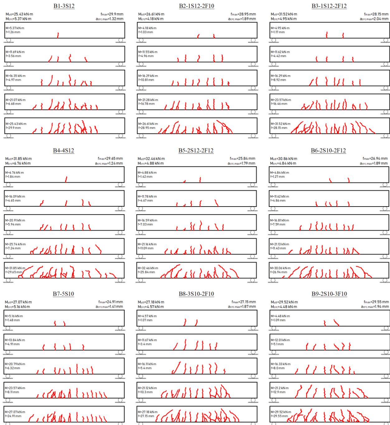
**Fig. 8. Stages of formation and development of cracks in beams under load**
