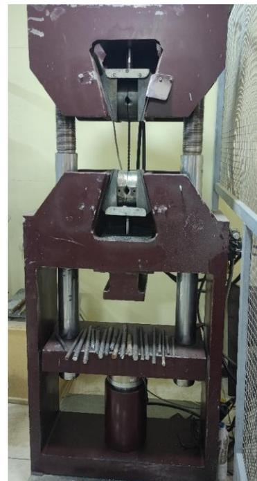
**Fig. 3. Testing steel bar**
