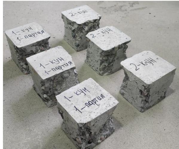
**Fig. 6. Tested cube samples**
