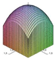
Since the base of the beam is a square with sides parallel to the coordinate axes Ox and Oy, the integration limits for both variables are constant.
