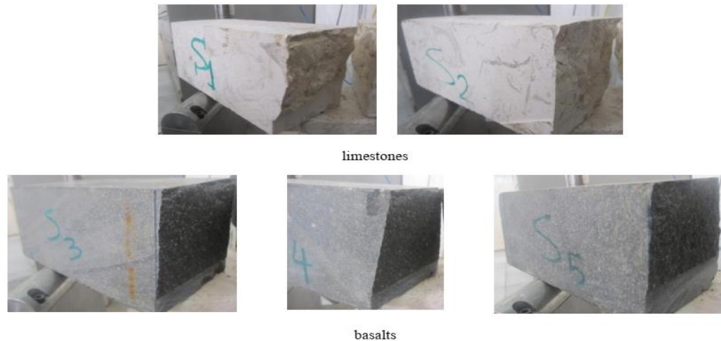
Fig.5: Fractured surfaces of limestones and basalts specimens under dynamic loading
