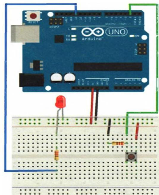
Рис 5: Wiring diagram for a LED controlled by a key
