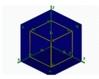
From point A, we omit the perpendiculars on the projection plane. The position of point A in space is determined by three coordinates (xA, yA, zA), showing the values of the distances by which the point is removed from the projection plane.
